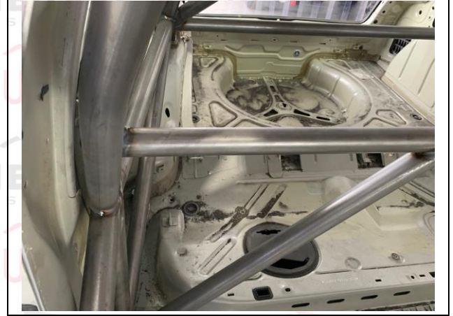
PHOTO 13 SHOULDER HARNESS ATTACHMENT - CO DRIVER
